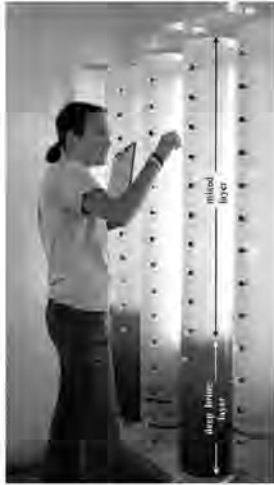
Fig. 2. Experimental columns used to test whether the presence of a deep brine layer increased mercury uptake of Artemia franciscana . Note the dark water of the deep brine layer in two of the tubes shown. For this image the plastic sheets covering the lower 50 cm of the tubes were removed.
